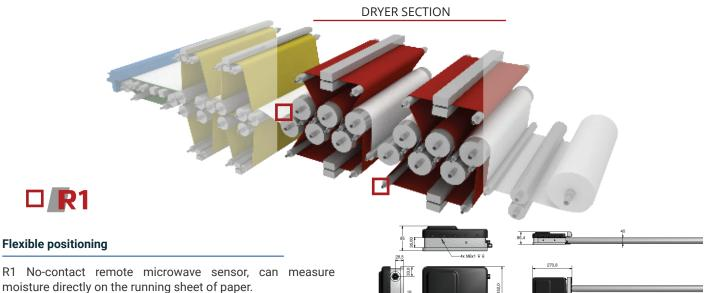
The R1 can be easily placed at the end of the press section or inside the dryer section with a proper cooling system.
